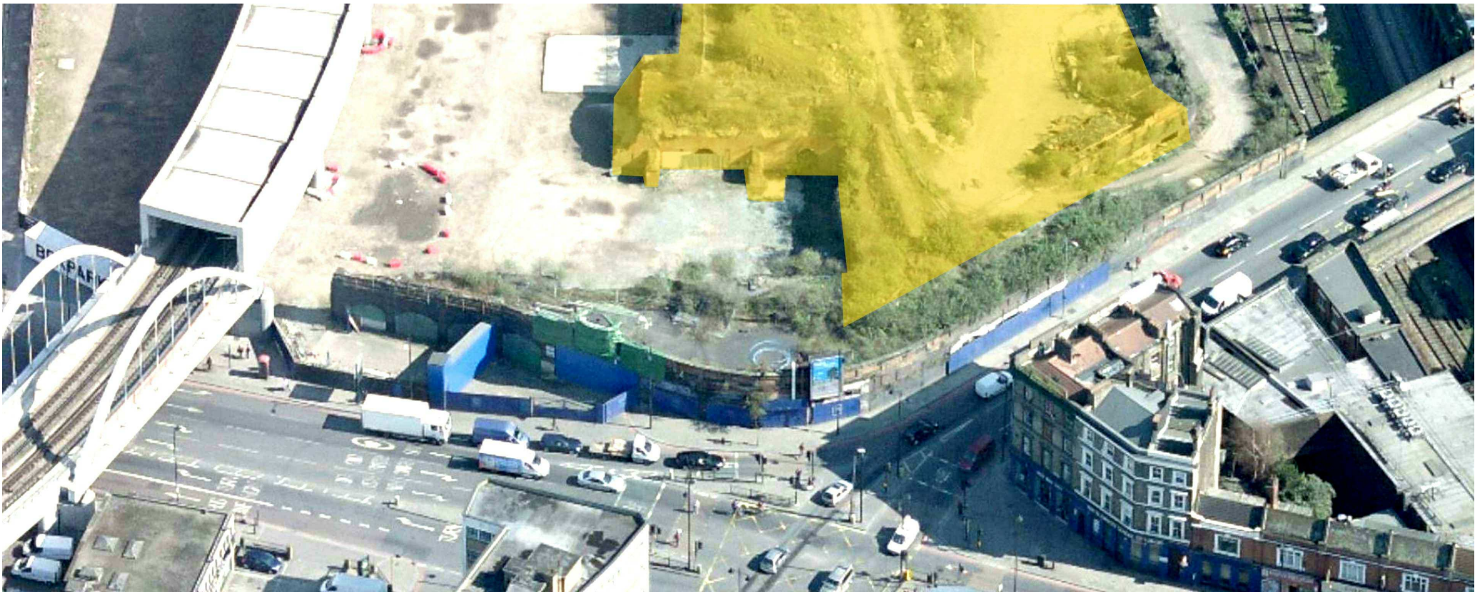
EXISTING BIRDS EYE VIEW FROM SOUTH WEST - Southern and Western Arches (highlighted yellow) are to be removed leaving the Oriel Gateway as a stand alone building.
